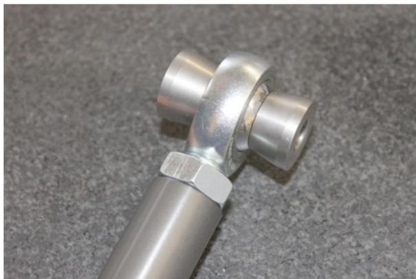
7. **NOTE:** Use wider stainless spacers on inside ball joint that attaches to sub-frame and the narrower stainless steel spacers on ball joint that attaches to outer suspension housing. The NM Control Arms have been pre-set to the factory length of 518mm (20.39").
