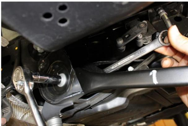
5. Unbolt and remove inner control arm bolt using E14 Torx or 11mm socket and 18mm wrench.
